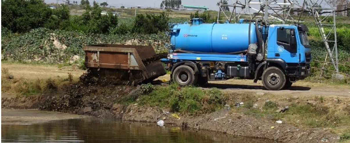
Figure 15 Emptying of septage from 6m3 AAWSA vacuum truck in Kotebe pond after being sieved in a metal container type screen (Source: field visit WWX, 1 November 2021)
