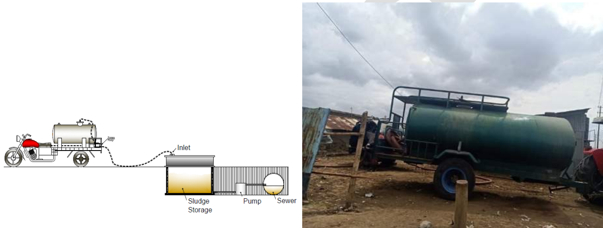
Figure 27 View of 2 transfer stations. On the left, a septic discharge station connected to the sewer (Source: MottMacDonald), on the right a 10m 3 tank mounted on a chassis in Nakuru (Source: WWX).
