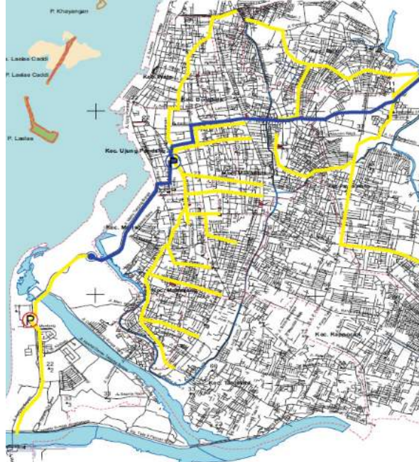
Figure 6.6: Potential Trunk Main Layout (Switch point)
