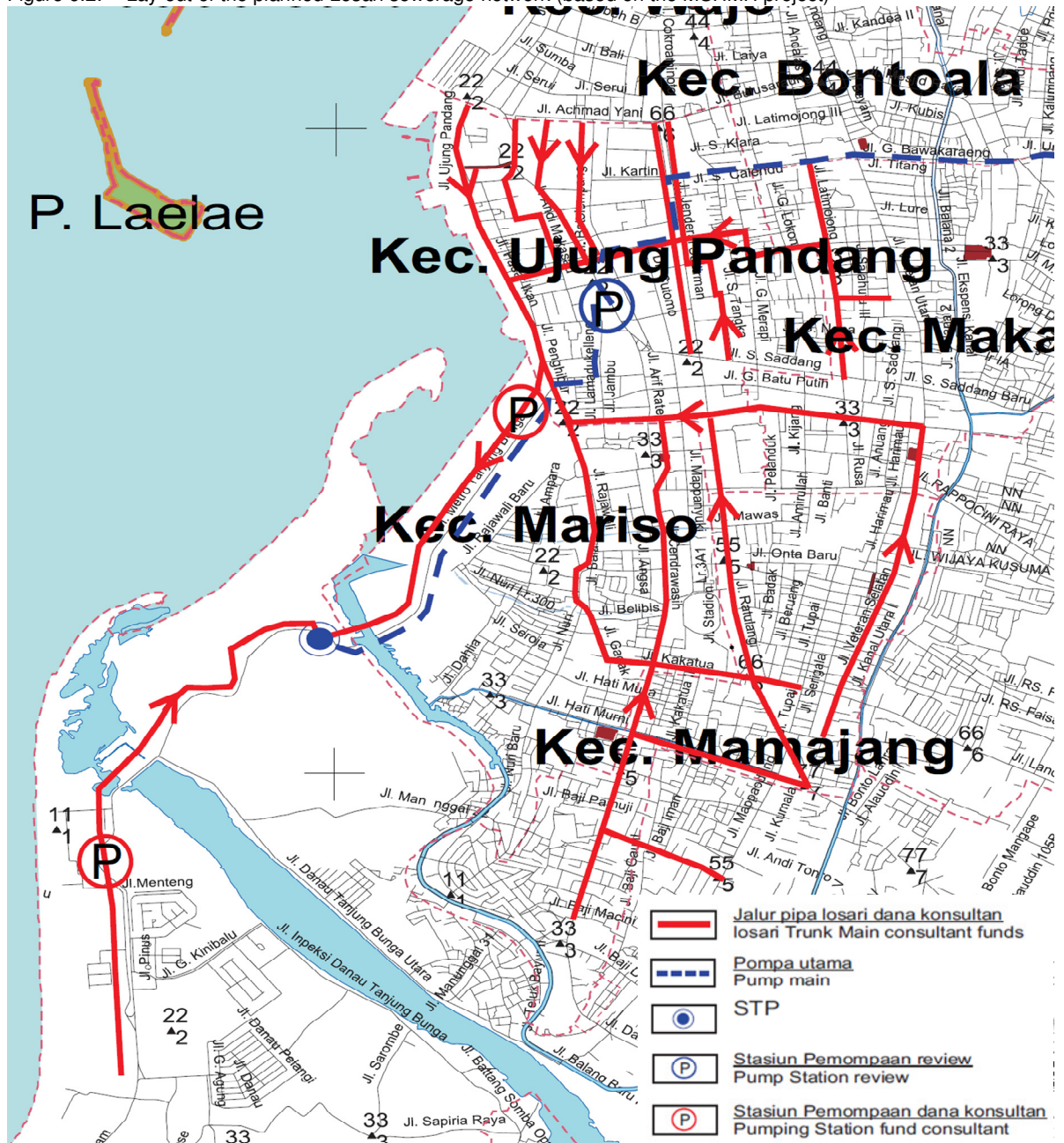
Figure 6.2: Lay-out of the planned Losari sewerage network (based on the MSHMH project)
