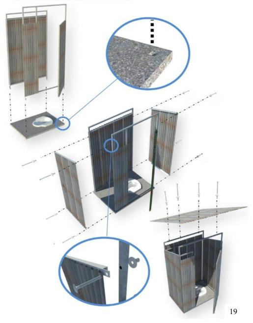
Ad b. Introduce plastic or Glass reinforced cement (GRC) sidewalls At present there are many easy to clean non-corrosive materials available for the shelter. Figure 5-5 illustrates the materials used in the SHAW project by Yayasan Dian Desa. Figure 5-5: Superstructure latrine, Yayasan Dian Desa (SHAW/Spit, 2011)
