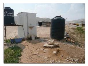
Additional difficulties are encountered in areas of hard bedrock or poor accessibility that prevent access for tankers to dislodge or construct large cesspits. Such designs although successful in their attempt to circumvent the restrictive planning rules and adapt to the hard physical environment are unsustainable in their longevity and offer poor environmental protection measures.
