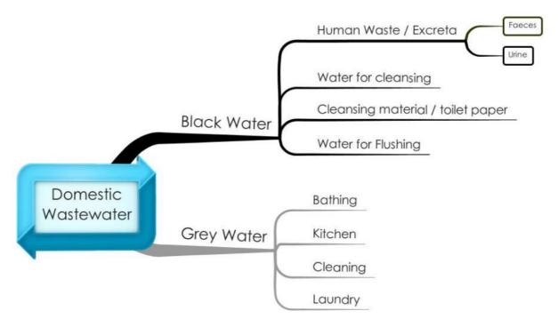
Domestic wastewater comprises all sources of liquid household waste: black water and grey water; see Figure 2-1 and Figure 2-2. However, it generally does not include storm water. **Storm water** in a community settlement is runoff from house roofs, paved areas and roads
