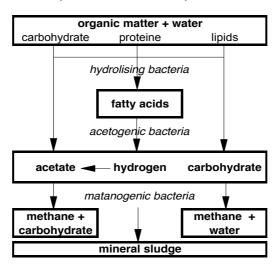
Principle of the anaerobic process
