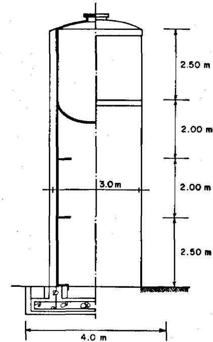
Fig. 10. The improved design. The structure resembles a bamboo.
