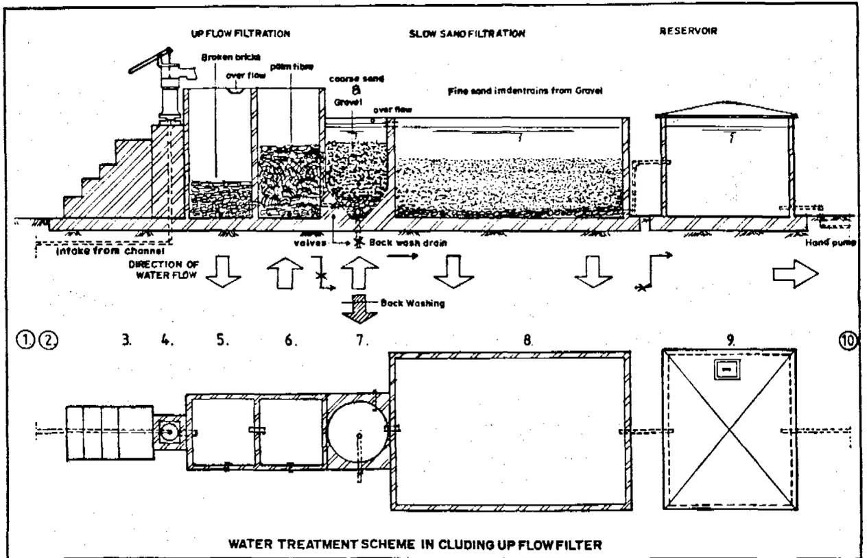
WATER TREATMENT SCHEME INCLUDING UP FLOW FILTER
